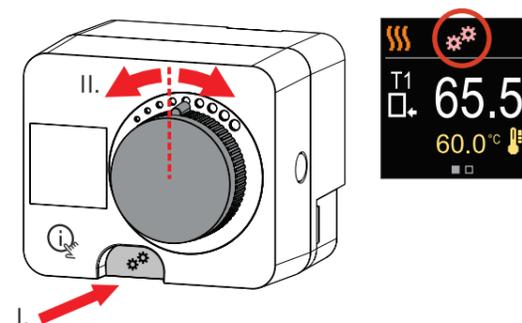
**i** When the clutch is activated, the control of the mixing valve switches off. The clutch symbol appears on the display.
