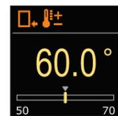
With the buttons  $\ominus$  and  $\oplus$  you can determine the requested temperature in heating mode. Confirm the setting with the  $\odot$  button. If you accidentally selected the wrong requested temperature, you can return to the requested temperature selection with the  $\odot$  button.
