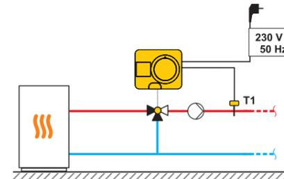
Scheme 2 - Control of supply - cooling
