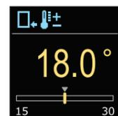
With the buttons  $\ominus$  and  $\oplus$  you can determine the requested temperature in cooling mode. Confirm the setting with the  $\odot$  button. If you accidentally selected the wrong requested temperature, you can return to the requested temperature selection with the  $\odot$  button.
