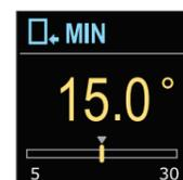
With the buttons  $\ominus$  and  $\oplus$  you can determine the lower limit setting of the requested temperature in cooling mode. Confirm the setting with the  $\odot$  button. If you accidentally selected the wrong lower limit, you can return to the lower limit selection with the  $\odot$  button.
