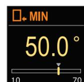
With the buttons  $\ominus$  and  $\oplus$  you can determine the lower limit setting of the requested temperature in heating mode. Confirm the setting with the  $\odot$  button. If you accidentally selected the wrong lower limit, you can return to the lower limit selection with the  $\odot$  button.
