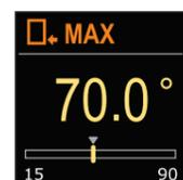
With the buttons  $\ominus$  and  $\oplus$  you can determine the upper limit setting of the requested temperature in heating mode. Confirm the setting with the  $\odot$  button. If you accidentally selected the wrong upper limit, you can return to the upper limit selection with the  $\odot$  button.
