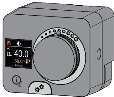
Controllers 1049-P230V are modern designed, microprocessor-driven devices made with digital and SMT technology. The controller is provided as a constant temperature controller with actuator designed for heating and cooling applications. The most common use is to control the return temperature in the boiler and the stand-pipe temperature in the system.
