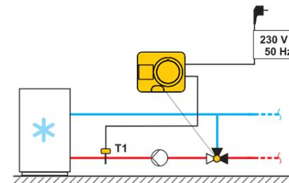
Scheme 2 - Control of supply - heating
