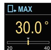
With the buttons  $\ominus$  and  $\oplus$  you can determine the upper limit setting of the requested temperature in cooling mode. Confirm the setting with the  $\odot$  button. If you accidentally selected the wrong upper limit, you can return to the upper limit selection with the  $\odot$  button.
